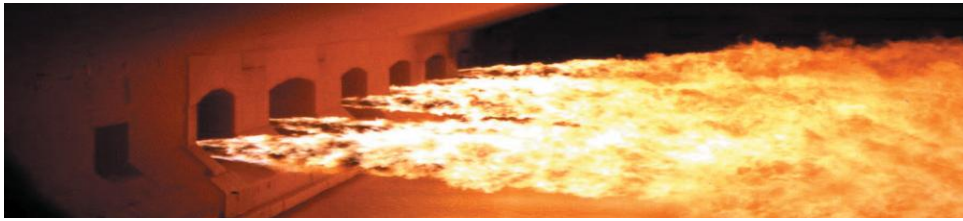
Figure 21 Gas heater of a float plant to melt the raw materials before the float process
